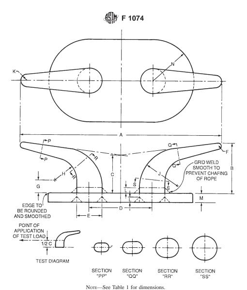
FIG. 1 Welded Horn Type Cleat (16 in.)
